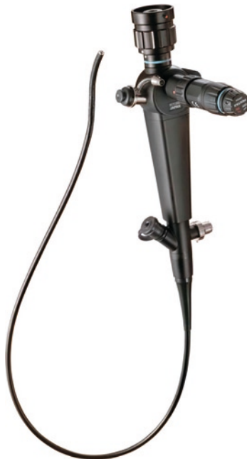
Fig. 11.13 A portable intubating scope manufactured by Pentax. Unlike the digital scope in Fig. 11.12, this scope has an eyepiece and a flexible, coherent light bundle in the insertion tube. The image is transmitted optically to the eyepiece through the coherent fiberoptic bundle. The control handle has an attached battery pack and light source making the scope portable (with permission Pentax Medical Company)
