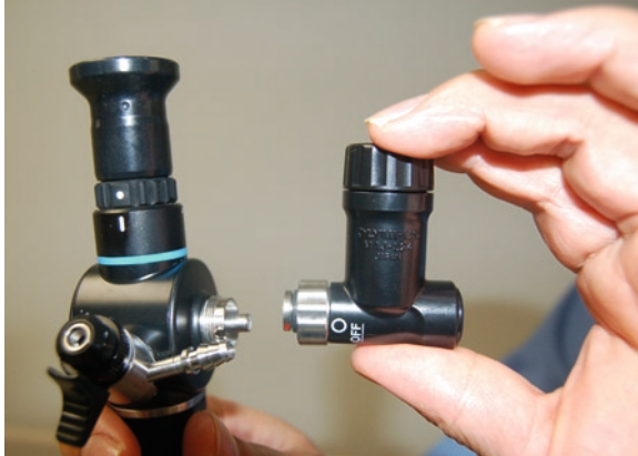
Fig. 11.11 A battery pack – On–Off switch ( right ) is attached to a portable fiberoptic scope
