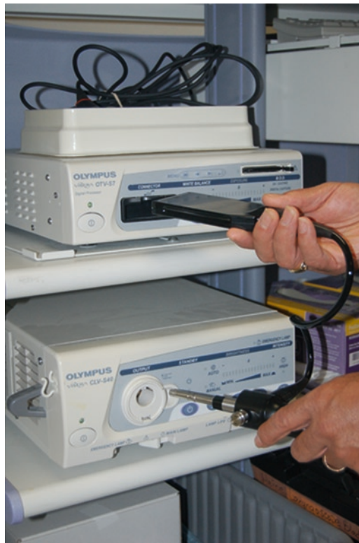
Fig. 11.10 The light cable ( lower ) from the fiberoptic scope is plugged into the light source. Digital systems have a second connection ( upper cable ) for the video connection
