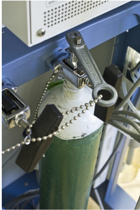
Fig. 4.6 The tank wrench used to open an E cylinder
